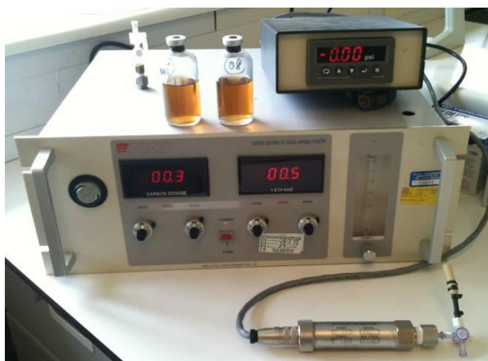
Figure 3 Gas analysis equipment and two incubation bottles for the gas production technique
